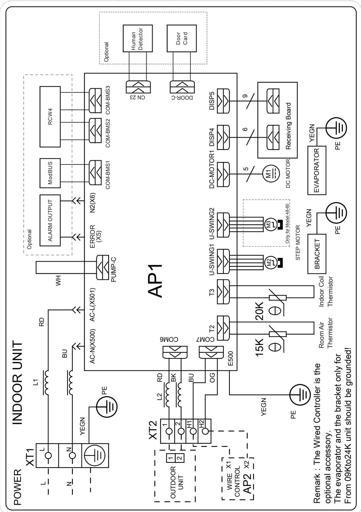
Remark : The Wired Controller is the optional accessory. The evaporator and the bracket only for From 09Kto24K unit should be grounded!
